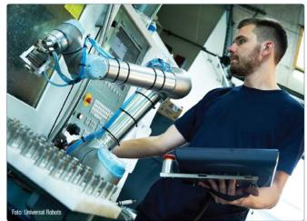
The robots are able to handle payloads of 5 kg (11 lbs) and 10kg (22 lbs) at a net mass of 18 kg (40 lbs) and 25kg (55 lbs). The lightweight robots can be easily moved between different work stations within a production facility and ships with easy-to-use software that allows a customer to be up and running in a few hours.
