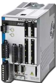
[AKD® BASIC](#) provides all the performance features from the AKD series, along with built-in machine and motion control that can be programmed in BASIC programming language from Kollmorgen's AKD WorkBench.
